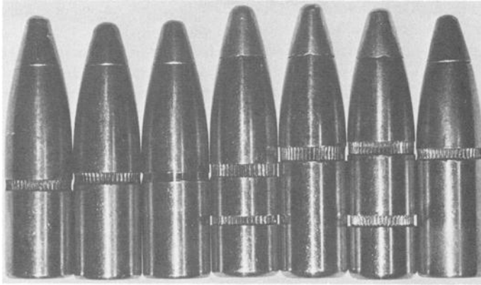
FIG. 8—"Silver-tip" bullets, 180 grain and 0.308 in. diameter, removed from (left to right) .30-40 Krag, .300 Savage, .300 Savage, .308 Winchester, .30-06, .30-06, and .300 H & H Magnum cartridges.
